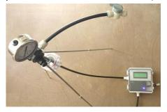
Power: The SDIcube<sup>TM</sup> is powered by either opening the enclosure and turning on the battery  $("I")^1$  or by plugging in the pump transformer that is provided with the optional SDIpump<sup>TM</sup> into its lower-right external power connection. The SDIpump<sup>TM</sup> is directly powered by the SDIcube<sup>TM</sup> by aligning their red and black wire connectors and initiating its operation with the black on/off button.
