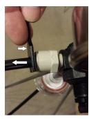
Press SDI3-in-1Tool<sup>TM</sup> against quick-connect fitting to release and pull out the 3/8" tubing
