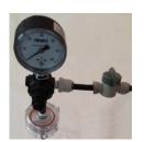
Includes: Manual SDI test assembly with pressure gauge and
